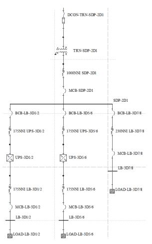
Figure 137: SDP-2D1 and loads one-line diagram.
