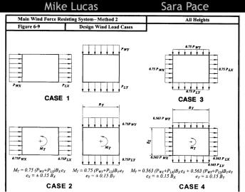
Figure 187: ASCE7-05 Figure 6-9 – MWFRS Wind Load Application.
