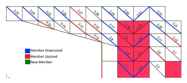
Figure 68: Cantilever Truss Redesign, Col Line 2.
