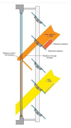
Figure 15: AWV Solar Shading Device Section.
