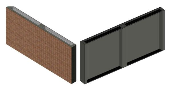
Figure 12: Redesigned Precast Panel (black indicates location of non-structural horizontal grating)
