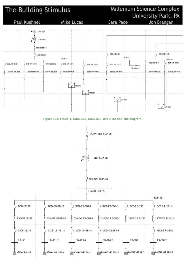
Figure 135: SDP-2B and loads one-line diagram.
