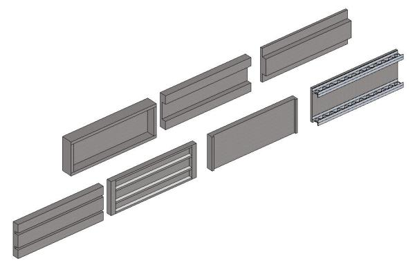
Figure 11: Precast Panel Iterations
