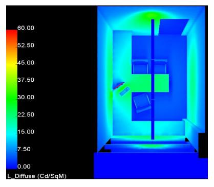
Figure 53: Typical Office - Luminance Color (Half Luminaires On).
