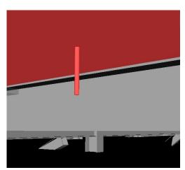
Figure 100: 2nd Floor Light Fixture Clash.
