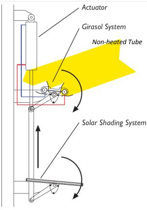
Figure 16: Girasol Shading Control.
