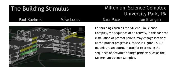
Figure 97: Precast Panel 4D Model.
