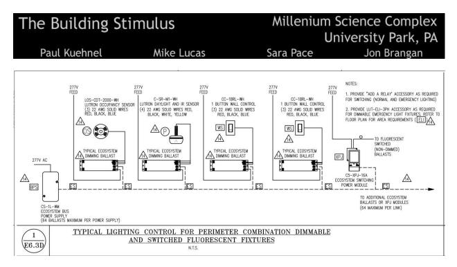
Figure 31: Existing Dimming Wiring Diagram.
