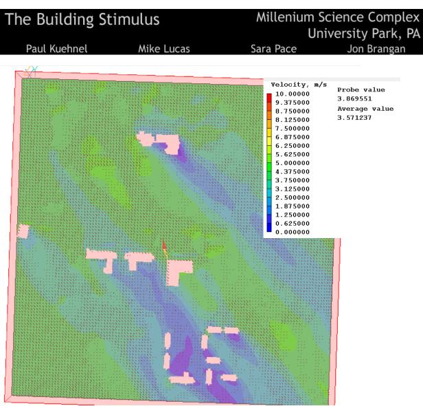
Figure 179: Z-Plane Velocity Profile: Z=24 m, Probe Position: (500, 430, 24)
