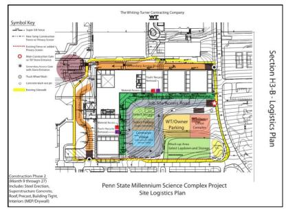
Figure 3: Phase Two Site Logistics Plan.
