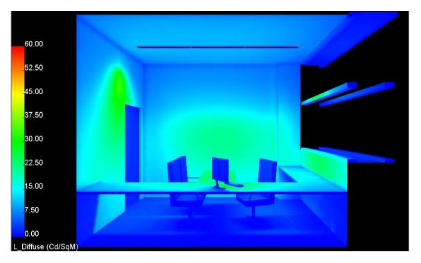
Figure 49: Typical Office - Luminance Color (Half Luminaires On).
