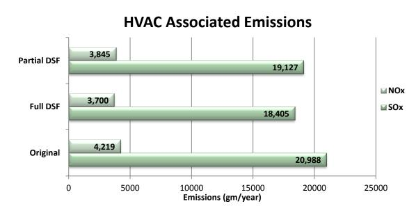
Figure 22: HVAC Associated Emissions for the 3rd Floor.
