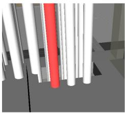
Figure 99: Conduit/Floor Slab Clash.
