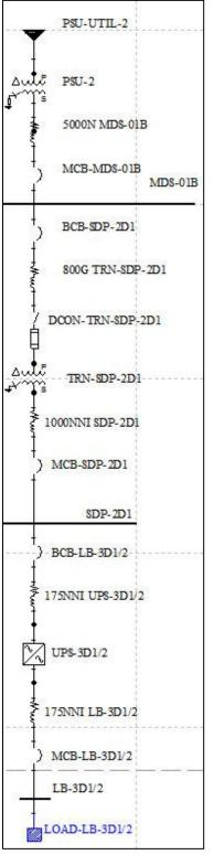
Figure 144: Short Circuit Analysis Path.
