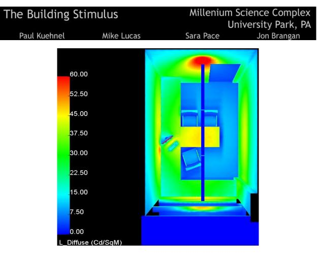
Figure 52: Typical Office - Luminance Color (All Luminaires On).
