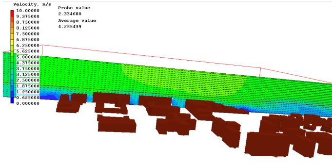
Figure 182: X-Plane Velocity Profile, Probe Location (500, 430, 10)
