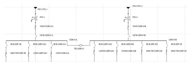
Figure 133: MDS-01A and MDS-01B one-line diagram.
