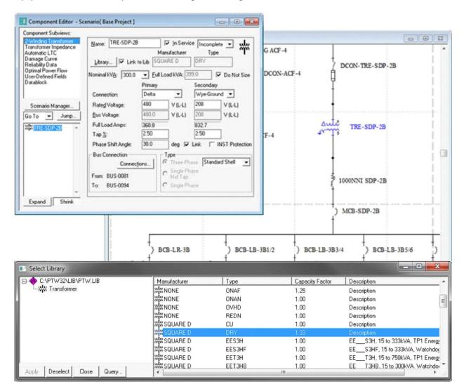
Figure 129: Transformer Inputs in SKM.
