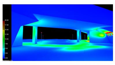
Figure 91: Exterior Plaza Lighting Design - Perspective View from South of Bridge (Color: Illuminance).
