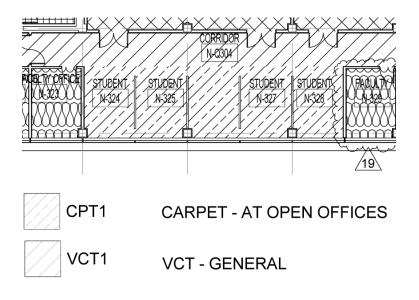
Figure 24: Corridor/Study Area Finish Floor Plan.
