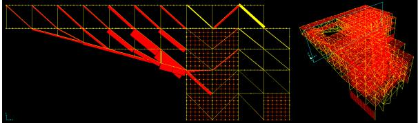
Figure 65: Existing Cantilever Truss Col Line 2.
