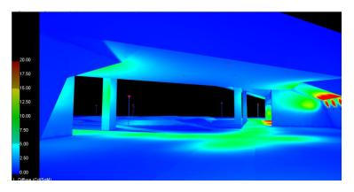
Figure 90: Exterior Plaza Lighting Design - Perspective View from South of Bridge (Color: Illuminance).
