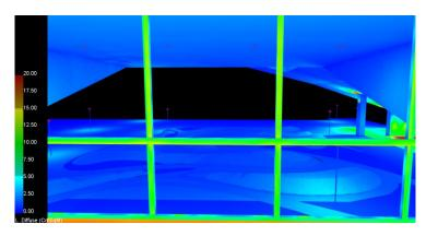
Figure 85: Exterior Plaza Lighting Design - Perspective View from 2nd Floor (Color: Luminance).
